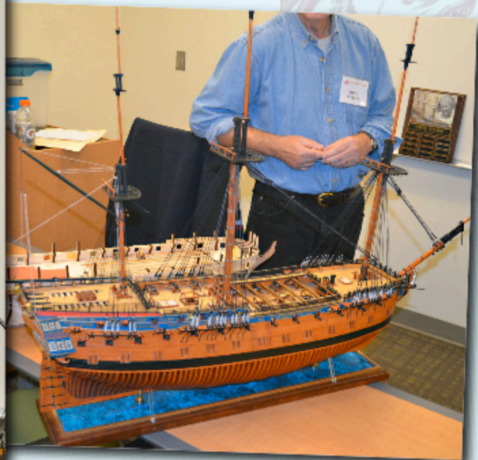
The large model's lower shrouds and mainstays are nearly done. Soon, a patient Dr. Goldberg will discover the "The Under-appreciated Joys of Making Scores of Ratlines."
